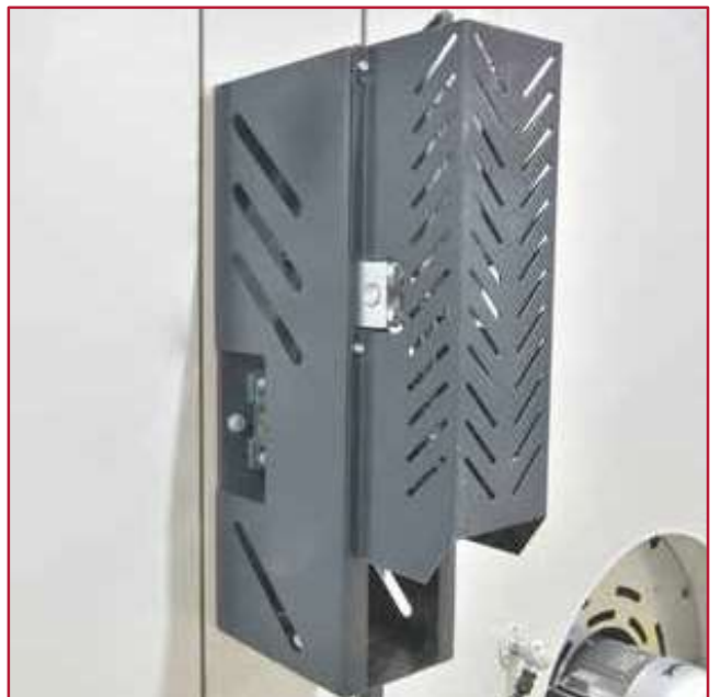
Pistonlu Tip Klepe Sistemi / Piston Type Flap System Devices for automatic control of air passage inside the suction filters
