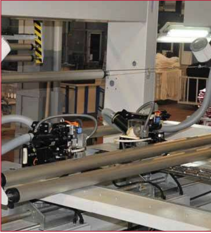
Çıkış Grubu Exit Unit working with tension control via load cells and voltage-free with low tension
