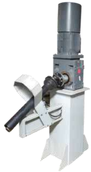
Merkez Tahrikli Dog Sarma Sistemi Big Batch Winding System with Central Drive
