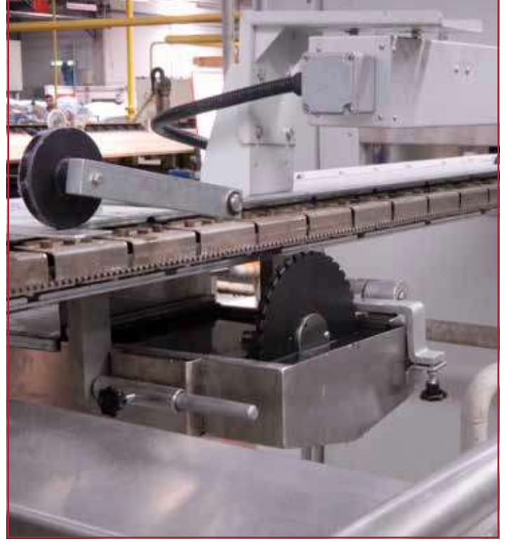
Kenar Kotalama Sistemi Alt Standart Gluing System
