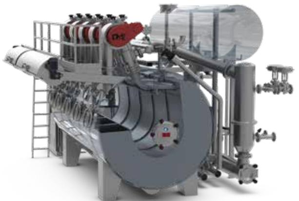
Ana pompa, Otomatik filtre, Eşanjör tesisatı / Main pump, Automatic filter, Heat exchanger installation
